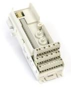
The TU811V1 is a 8 channel 250 V compact module termination unit (MTU) for the S800 I/O. The MTU is a passive unit used for connection of the field wiring to the I/O modules. It also contains a part of the ModuleBus.
