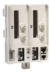
The TU846 is a module termination unit (MTU) for redundant configuration of the field communication interface CI840/CI840A and redundant I/O. The MTU is a passive unit having connections for power supply, two electrical ModuleBuses, two CI840/CI840A and two rotary switches for station address (0 to 99) settings.
