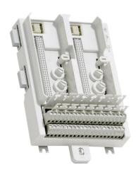
The TU844 MTU can have up to 8 I/O channels and 2+2 process voltage connections. Each channel has two I/O connections and one ZP connection. Input signals are connected via individual shunt sticks, TY801. The shunt stick is used to choose between voltage and current input. The maximum rated voltage is 50 V and maximum rated current is 2 A per channel.
