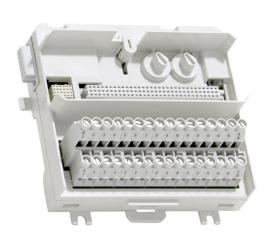
The TU851 MTU can have up to 16 I/O channels. The maximum rated voltage is 250 V and maximum rated current is 3 A per channel. The MTU distributes the ModuleBus to the I/O module and to the next MTU. It also generates the correct address to the I/O module by shifting the outgoing position signals to the next MTU.
