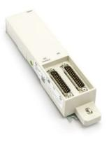
The TB846 redundant ModuleBus Cable Adaptor is used together with TB845 and two TK801V0xx to extend the ModuleBus. Using this extension I/O modules on the same electrical ModuleBus can be mounted on different DIN rails. TB846 can also be used together with TB842 to provide an optical extension of the ModuleBus.
