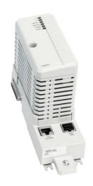
The CI873A is an AC 800M communication interface that connects to external Ethernet devices using the EtherNet/IP protocol. The TP867 Baseplate has two RJ45 Ethernet connectors, but only the CH1 connector that supports 100Mbps is used. The CI873 expansion unit contains the CEX-Bus logic, a communication unit, and a DC/DC converter that supplies the required voltage from +24 V supply through the CEX-Bus.
