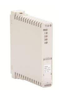
The remote S900 I/O system can be installed in non-hazardous areas or directly in Zone 1 or Zone 2 hazardous area depending on the selected system variant. S900 I/O communicates with the control system level using the PROFIBUS DP standard. The I/O system can be installed directly in the field, therefore the costs for marshalling and wiring are reduced.
