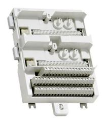
The TU843 MTU can have up to 16 I/O channels and 2+2 process voltage connections. Each channel has two I/O connections and one ZP connection. The maximum rated voltage is 50 V and maximum rated current is 3 A per channel.
