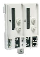
The TU847 is a module termination unit (MTU) for redundant configuration of the field communication interface CI840/CI840A. The MTU is a passive unit having connections for power supply, electrical ModuleBus, two CI840/CI840A and two rotary switches for station address (0 to 99) settings. A ModuleBus Optical Port TB842 can be connected to TU847 via TB806.
