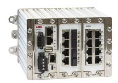
NE820 is an Industrial switch made for harsh environments. Due to our multi-rate SFP solution, the switch can be used in either 100 Mbit or Gigabit networks. Our unique FRNT (Fast Recovery of Network Topology) technology is the fastest protocol on the market to re-configure a network in case of any link or hardware failure. That is why NE820 is also used in safety-critical applications such as tunnels, traffic signal control, and railway systems.
